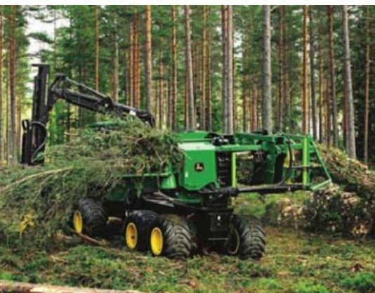
Specialized equipment can bundle logging waste for bioenergy applications. Photo courtesy John Deere.
