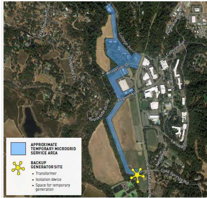
Figure 12: Approximate Energization Area of Angwin Temporary Microgrid
