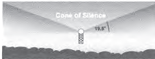
Figure 2 Illustration of the total elevation angle coverage of the radar
