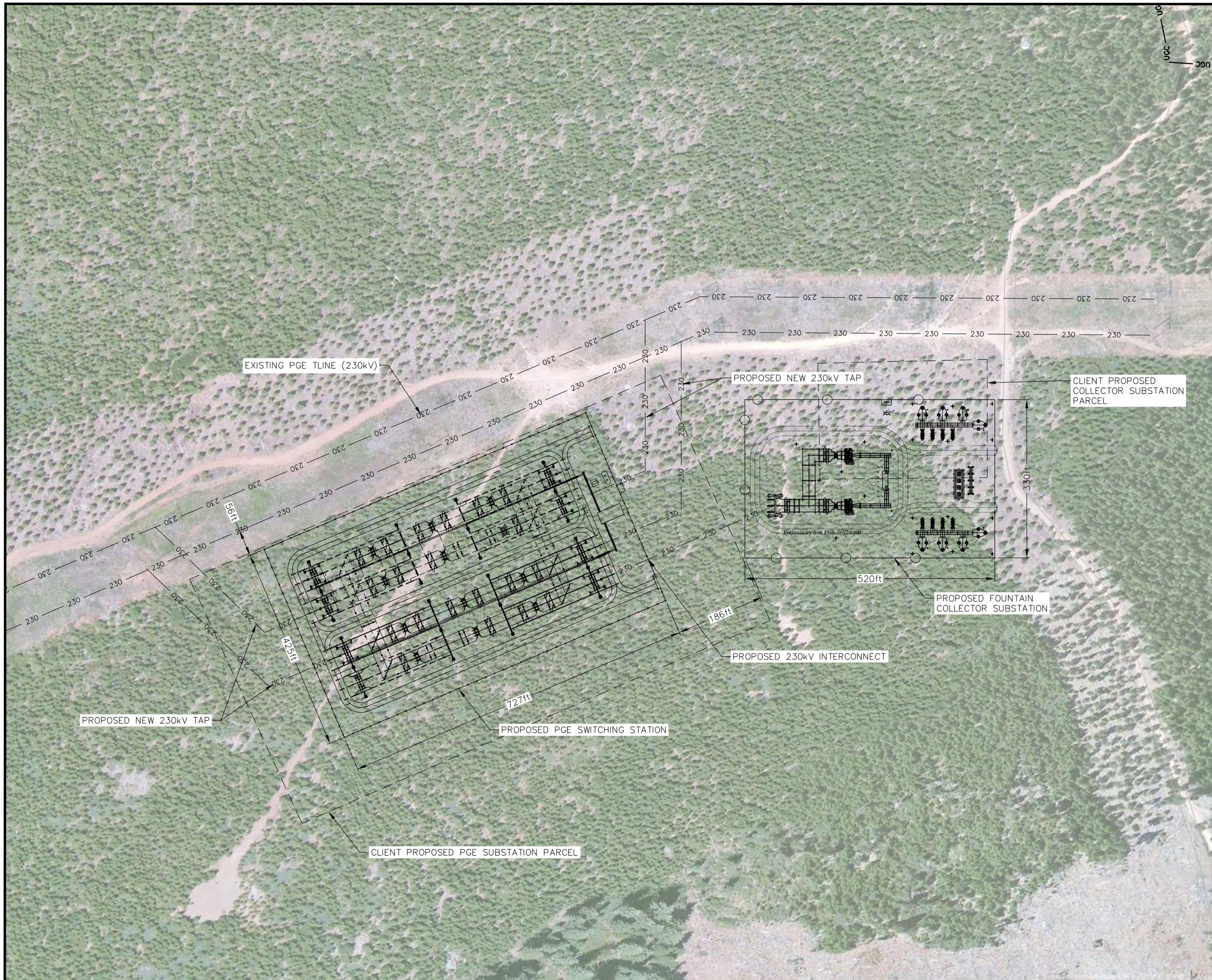
Figure 10: Site Plan Collector Substation and PG&E Point of Interconnect Switchyard
